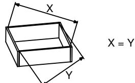
**Attention! The bottom of the drawer should be nailed after setting up the diagonal between the elements (see drawing).**
